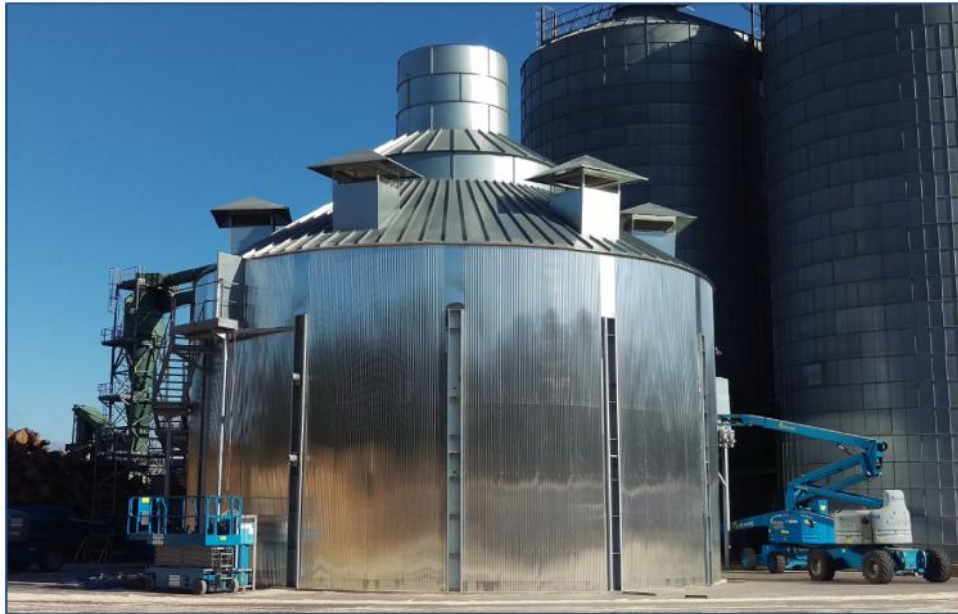
Figure 2: Dryer One drying machine for drying wooden sawdust.
