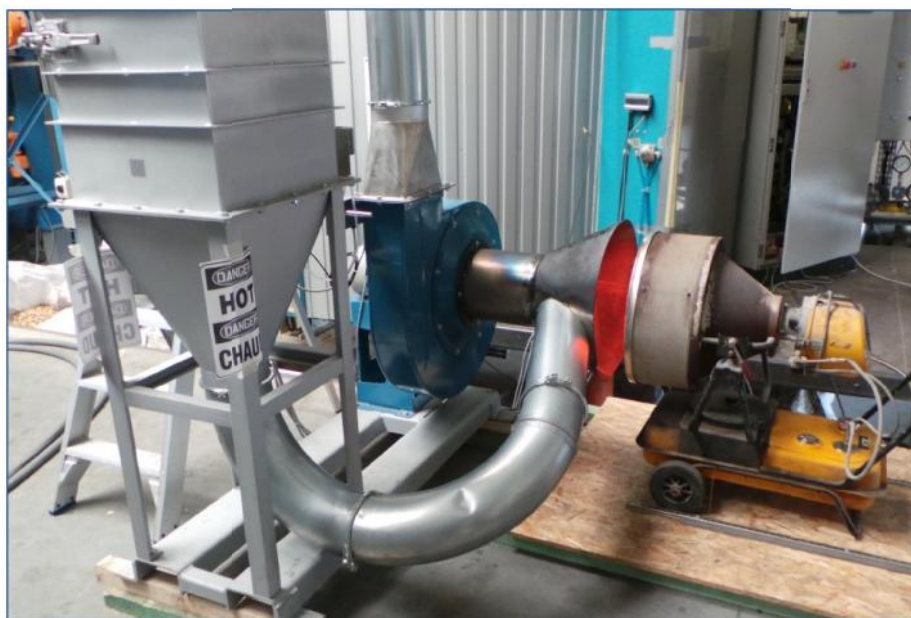
Figure 6: Adaptation for the recirculation of air in a closed circuit.
